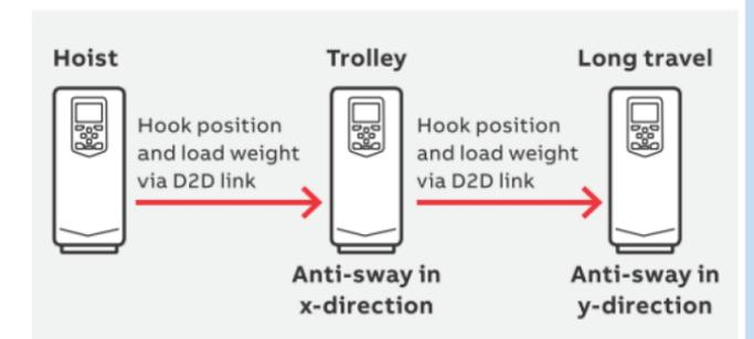
The drives communicate with each other via a D2D link. The hook position can also be transmitted with fieldbus or analog communication.
