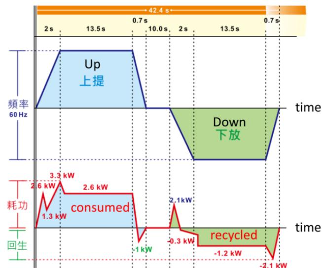
On a 10-ton crane, the lifting speed is 3.6 m/min, and a 5.5 kW motor is equipped with an electric energy feedback unit. When hanging 3 tons of goods, use power analyzer to compare the power saving rate of 5 times up and down.
